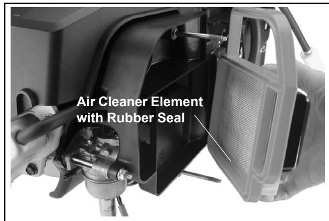
Figure 10. Removing Air Cleaner Element.
